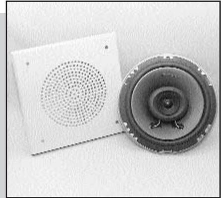
The **BSI - 90 Monitor Speaker** is a 2-way bass reflex speaker with a cast aluminum back-box and perforated steel grill. Well suited to surface mount and/or bookshelf-type indoor applications. 3-1/2" woofer, 2" soft dome tweeter, 20 watts continuous power, 8 impedance, 60-20kHz dynamic response. Measures 7-1/4"(w) x 4-1/2"(d) x 4-1/2"(h), matte black finish. 1 yr warranty, 7 lb shipping weight. Includes swivel mounting bracket, various mounting hardware, standard quick-connect terminals.
