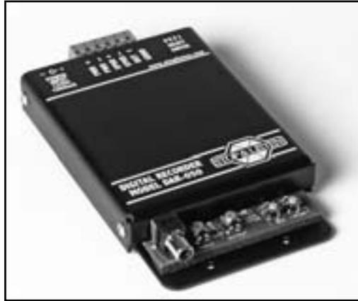
For continuous play or looping applications, connect a wire jumper between the external BUT button and GND ground terminals. The audio track will play to the end, then automatically reset to the beginning and start over. Remember that DIP#2 should be in the DOWN position and DIP#4 should be UP. (TIP - for a delay before the audio track repeats itself, simply leave a bit of blank space at the beginning or end of the audio track when making the recording.)
