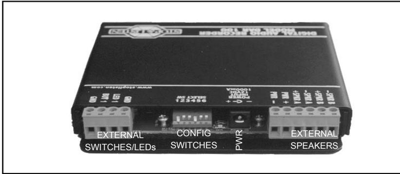
**RECORD LOCK-OUT FEATURE** The DAR-100 incorporates RECORD LOCKOUT features to prevent accidental erasure of the recorded message. In order to record a new audio track, an audio cord MUST be plugged in to the LINE IN jack or MIC jack, and Configuration Switch #3 (Record Enable) on the back of the unit must be in the UP position.
