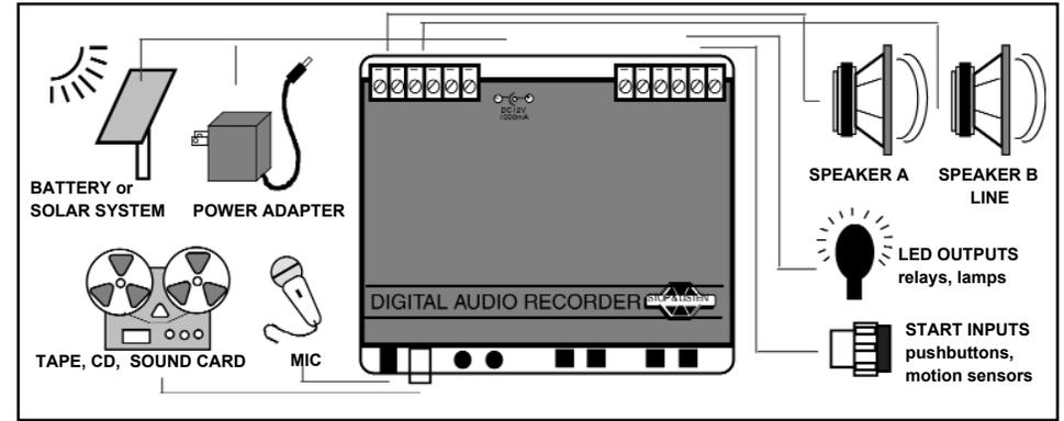
**POWER INPUT** - Plug the supplied wall-plug adapter in here. Requires 12 volt DC nominal, 800mA, center positive. Internally fused 1 amp type 2AG.
