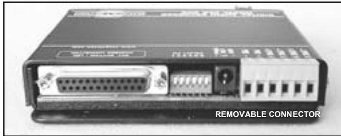
**MOUNTING** This unit can be mounted in any orientation. 4 mounting holes are provided, 2 on each end of the chassis (may require removal of orange connector block).
